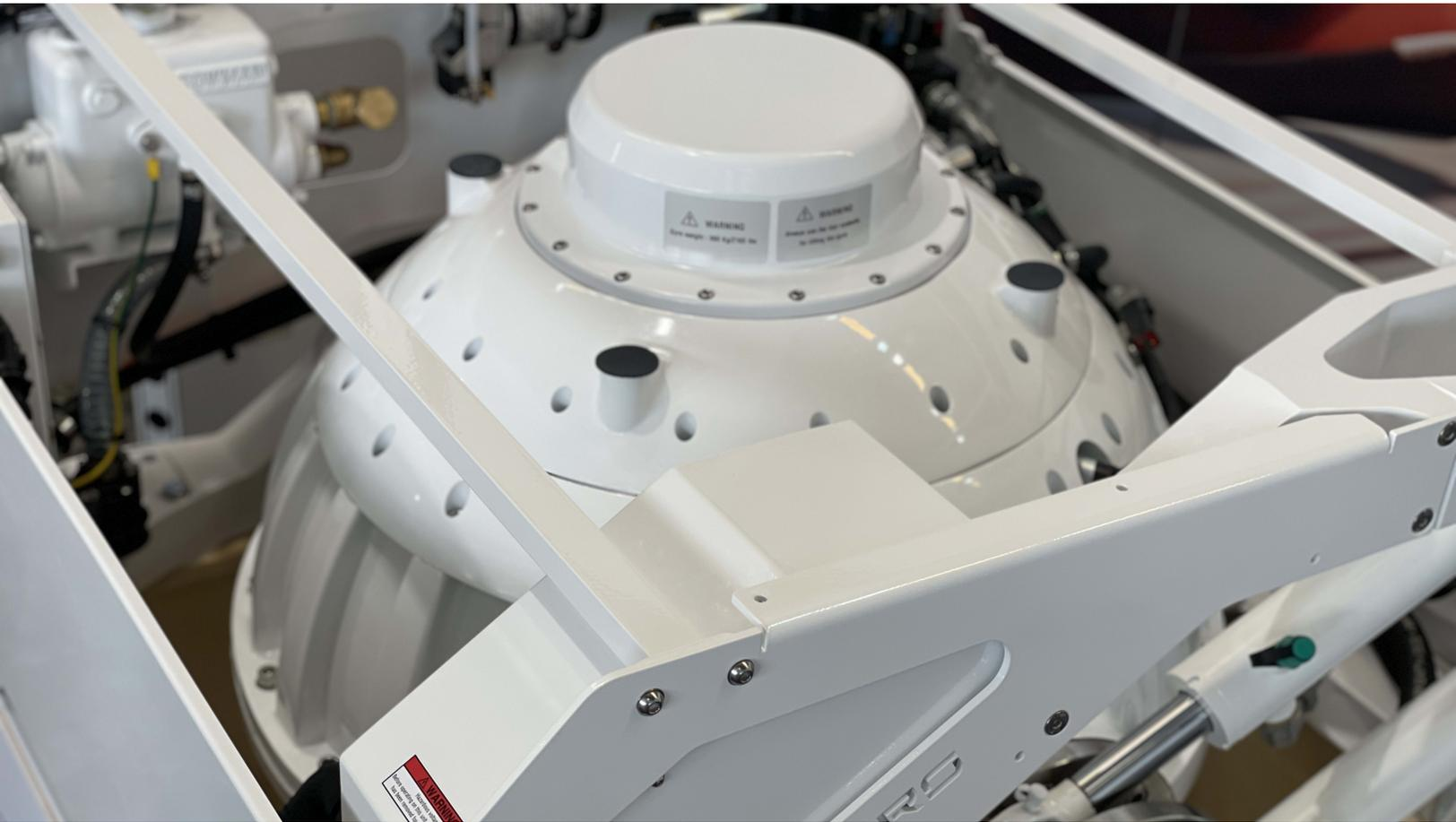
The new Smartgyro SG60 gyroscopic stabilizer for boats from 55 feet to 65 feet
